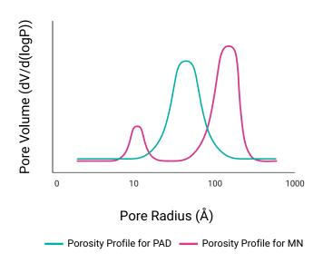
The higher proportion of small micropores in the range of 10–30 Å within Macronet adsorbents leads to:
